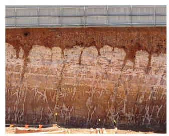
**Epikarst surface:** A *laterite karst* example. A detrital laterite soil overlies an irregular epikarst surface with grikes (*cutters*) and pinnacles. KG088054P. Excavation in city of Darwin, NT.
